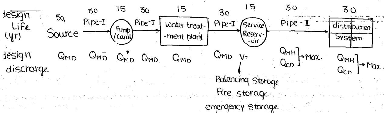
Q- A city with the population of 1.8 Lakh has per capita water demand of 300 lit/day. It is to be provided with the water supply scheme. Report the imp. type of demand of this water supply scheme & also indicate the design capacity of different components of this water supply scheme.
