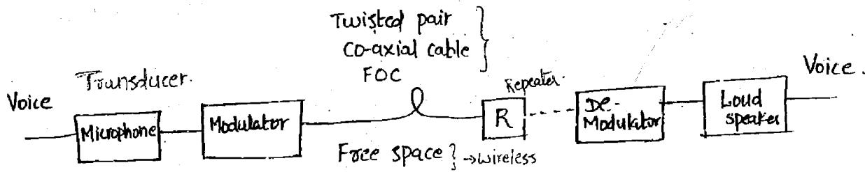
\* The no. of repeaters required in a communication link depends on the distance, type of the cable used, Txtd power, and type of modulation technique used.
