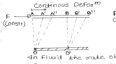
In fluid the rate of deformation is important
