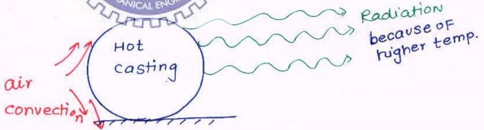
case:3 Hot<sup>molten</sup> Metal when poured in mould cavity:
