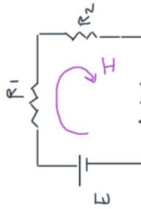
$$E = IR_1 + IR_2 + IR_3 \\ = I(R_1 + R_2 + R_3)$$
