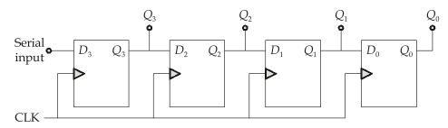
Input is given at  $D_3$  and output is taken from  $Q_3Q_2Q_1Q_0$
