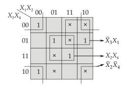
Simplified expression is  $X_2X_4 + \overline{X}_2\overline{X}_4 + X_1\overline{X}_3$
