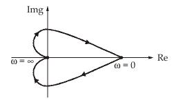
The obtained Nyquist plot of  $G(j\omega)$   $H(j\omega)$  does not encircle the (-1 + j0) point in  $j\omega$  plane for any positive value of a and b. Hence system is stable system.
