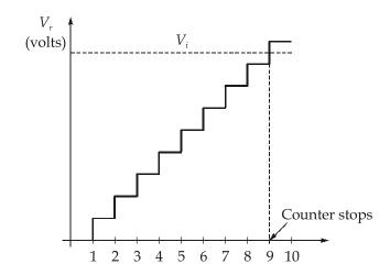
The counting will continue until the reference voltage  $V_r$  equals and just rises more than  $V_i$ . Then the comparator output becomes low and this disables the AND gate from passing the clock. The counting steps at the instance  $V_i < V_r$  and at that instant the digital output represents the analog input voltage  $V_i$ . Then the clock is inhibited, the counter stops its
