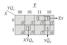
$T = \overline{X}Y + Y\overline{Q}_n + X\overline{Y}Q_n$
