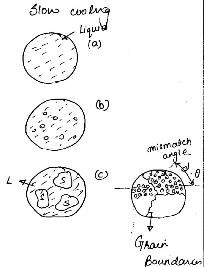
A sample of Cu and Ni, with  $60\% \text{ Ni}$ , is cooled slowly along line a-d and its micro-structure is observed. At point a entire sample will be in the liquid state and the moment temp of the sample slightly decreases below liquidus line to point b. Solid start nucleating in the microstructure. Upon dec. the temp slowly from point b to c following conclusions can be drawn by using the lever rule:
