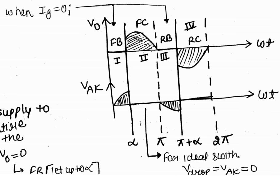
when we are not giving supply to gate terminal + then entire voltage appear across the switch. ( $V_{AK} = V_S$ ) &  $V_0 = 0$
