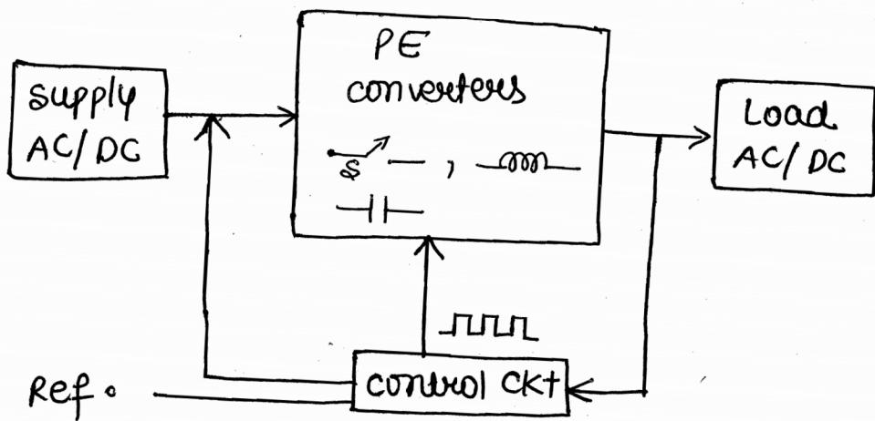
power electronic deals with control, conversion and conditioning of electric power using semiconductor devices & these sc devices should operate with high efficiency. In power electronic, semiconductor devices are mainly used as switches.
