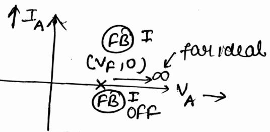
An ideal device when blocking the forward voltage ( $V_F$ ) then current passing through the device is zero Amp but in practical some leakage current flow through it due to minority current now, we are having some losses in semiconductor device even in the OFF state i.e.,  $\text{blocking power loss} = [V_F \times I_{\text{leakage}}]$ . If it is ideal switch then it can block  $\infty$  voltage through it. But practically it is not possible to apply  $\infty$  voltage across it.
