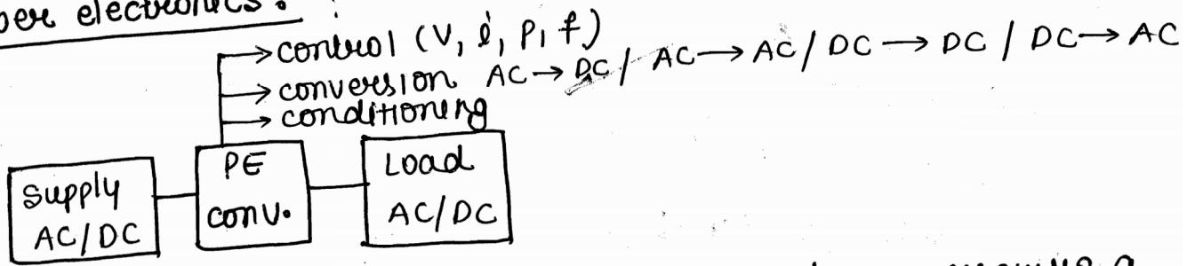
Due to the mismatching of power in both side we require a device which is known as power converters.
