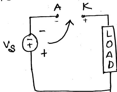
IV mode - Now, giving  $-I_g$  (negative pulse) signal to the TRIAC the TRIAC start conduction in reverse direction negative voltage appear across the load.
