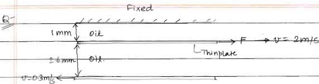
Thin plate has a plan Area of  $40\text{cm} \times 40\text{cm}$
