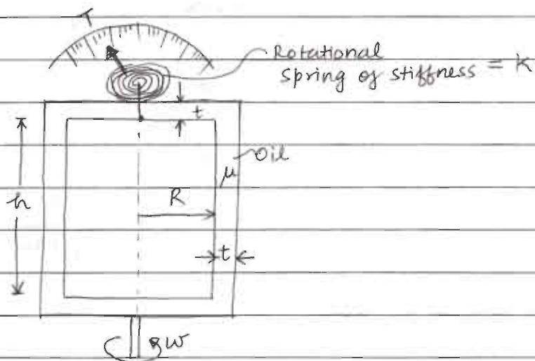
$$T_{\text{bottom}} = T_{\text{top}} = \frac{\pi \mu w R^4}{2t}$$
