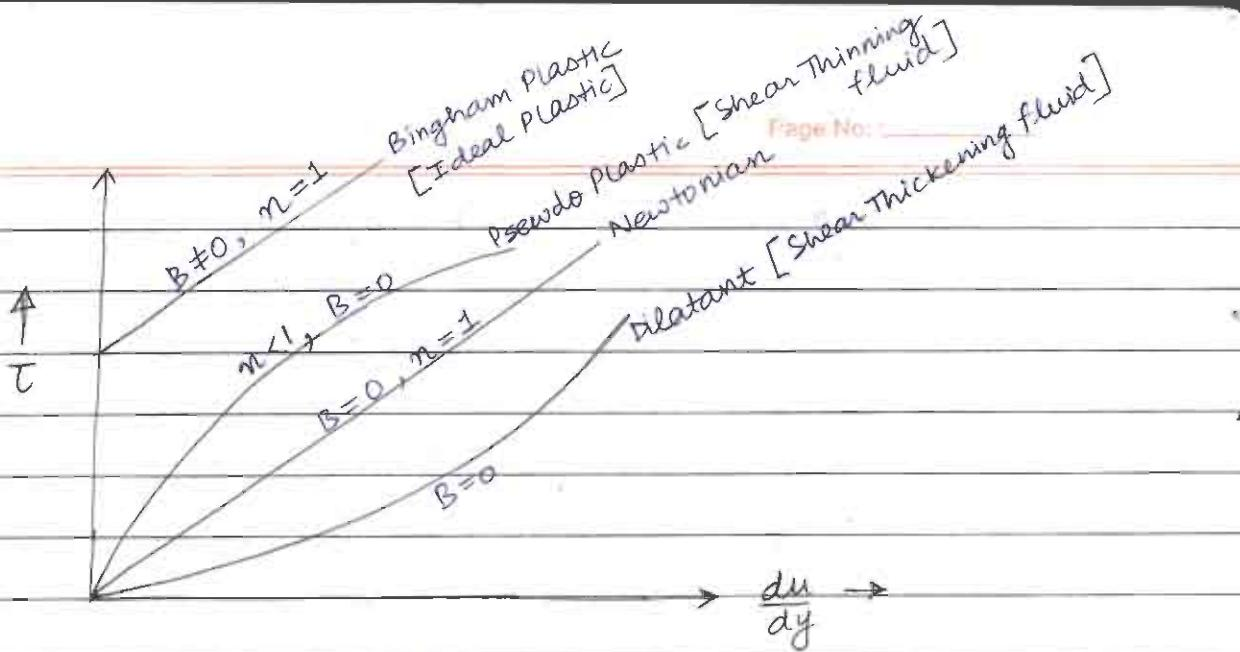
$$\frac{d(\tau)}{d(\frac{du}{dy})} = A n \left( \frac{du}{dy} \right)^{n-1} \Rightarrow \text{Apparent viscosity}$$
