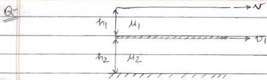
The top plate is being pulled with velocity  $v$  and the middle plate moves due to the pulling of upper plate with a uniform velocity  $v_1$  ( $v_1 < v$ ). Find the ratio of  $v_1/v$  with the assumption that the velocity variation b/w the plates is linear.
