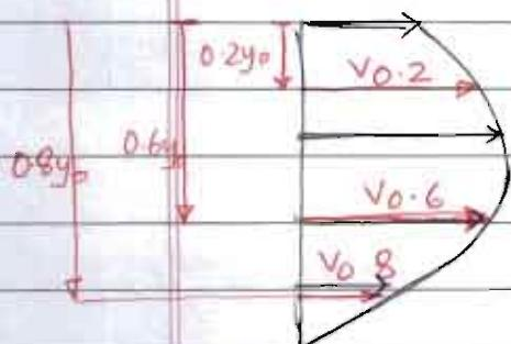
$$V_{\text{avg}} = V_{0.6} = \frac{V_{0.2} + V_{0.8}}{2}$$
