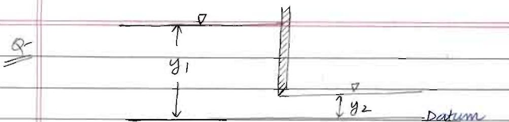
Find the force exerted by water on the sluice gate assuming negligible losses.
