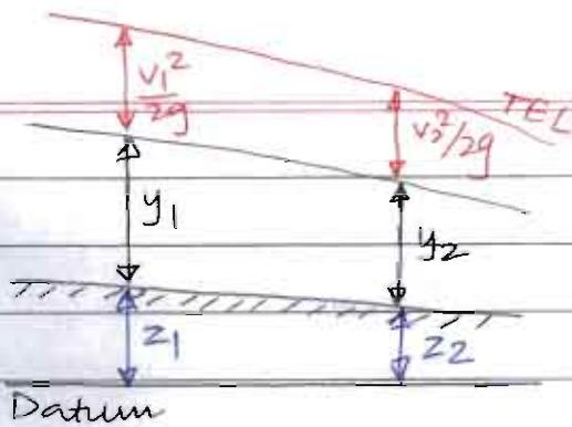
$$\frac{P_1}{\gamma} + z_1 + \frac{v_1^2}{2g} = \frac{P_2}{\gamma} + z_2 + \frac{v_2^2}{2g} + h_L$$
