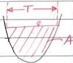
→  $c = \sqrt{gD}$  = celerity → velocity of small gravity wave that occurs in shallow water, generated due to disturbances or obstacles in the channel. It is the velocity of wave wrt water and travels both upstream and downstream.
