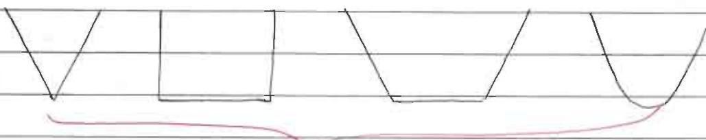
Only one normal depth of flow for a fixed  $Q, n, S_0$ .
