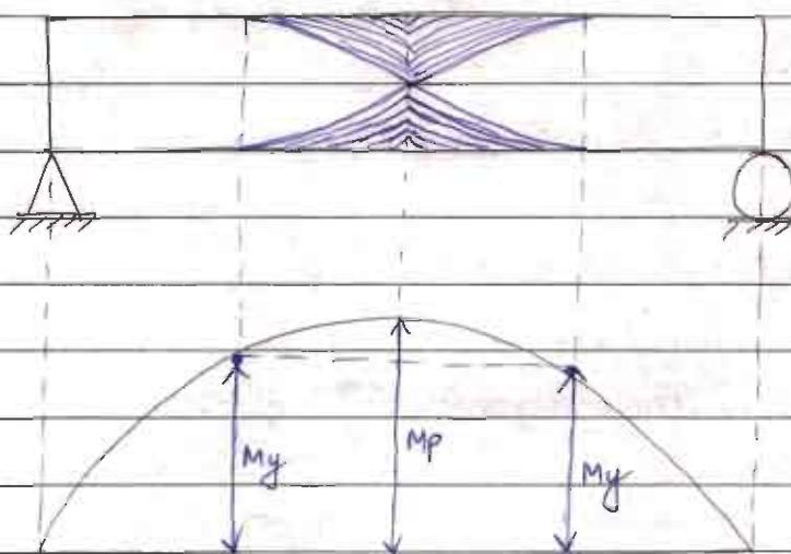
→ Plastic hinge can be defined as a yielded zone due to flexure in a structure in which infinite rotation can take place at a constant resisting Moment,  $M_p$  of that section.
