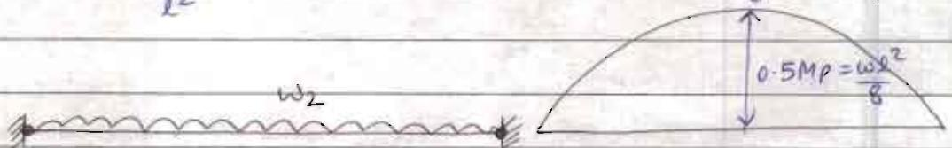
when  $w_2 = \frac{4MP}{l^2}$ , the mid-span will become a plastic hinge
