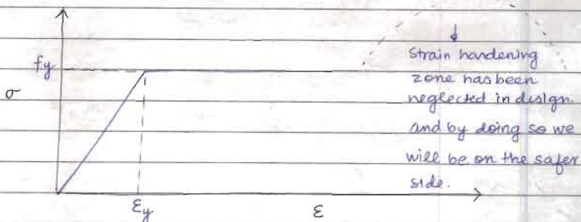
(4) Relation between stress and strain is same in tension and compression
