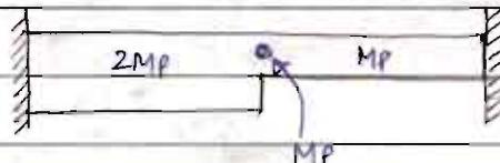
→ When 2 sections join at a point plastic hinge forms in the section of smaller  $M_p$ .
