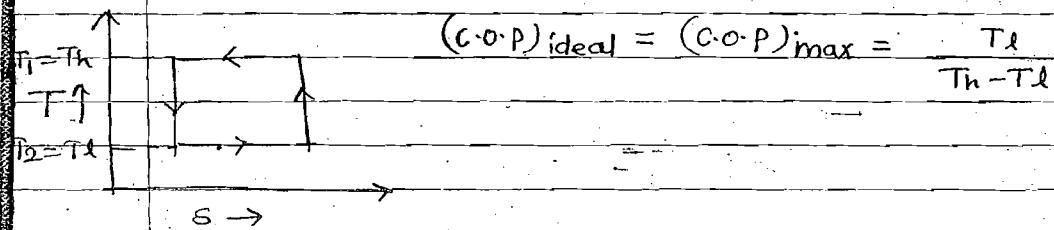
Note: lower temp is known as evaporator temp and higher temp is known as condenser temp.
