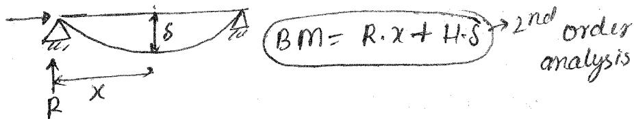
Note: If deformations are large, action of loading will be affected by deformation of structure.
