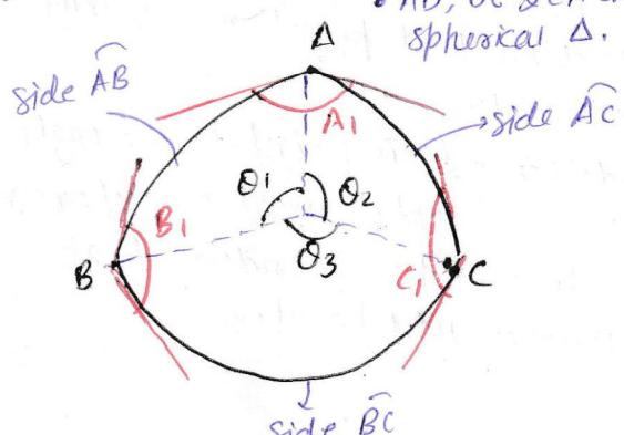
$\angle A, \angle B, \angle C \rightarrow$  spherical angle
