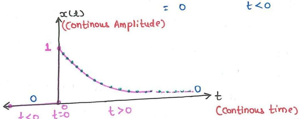
$$\begin{aligned} t=0 &\Rightarrow \text{Amplitude} = e^0 = 1 \\ t=\infty &\Rightarrow \text{Amplitude} = e^{-\infty} = 0 \end{aligned}$$
