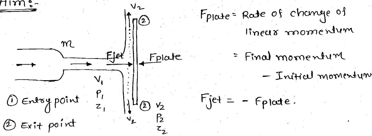
$$F_{\text{plate}} = \text{Rate of change of linear momentum}$$
