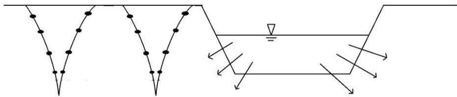
In this method (Artificial) water is supplied artificially direct into the rootzone with the help of network of pipe and draining it is termed as artificial sub-surface irrigation.
