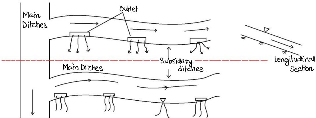
② BORDER FLOODING: In this method, land is divided into no. of strips, separated by low levees. {Note: Levees are small embankment, which don't permit the flow of water across it}
