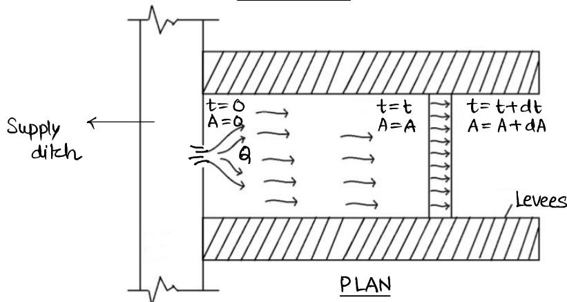
A relationship between the discharge through the Supply ditch, the average depth of water flowing over the Strip ( $y$ ), the rate of infiltration of Soil( $f$ ), the area of the Land irrigated ( $A$ ) and the approximate time required to cover the given area is Given by -
