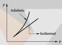
Bulk modulus is not constant and it increases with increase in pressure because at higher pressure the fluid offer's more resistance for further compression.
