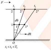
As long as there is a shear force fluid flows or deform continuously. Ex: liquids, gases, vapour etc.
