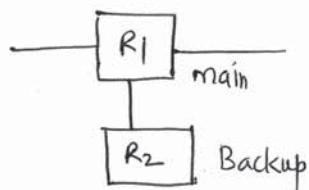
$$R_s = R_1 + R_2(1 - R_1)$$
