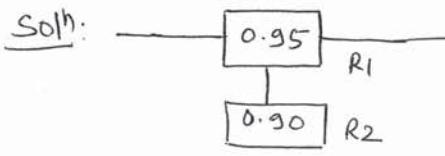
$$\begin{aligned} R_s &= R_1 + R_2(1 - R_1) \\ &= 0.95 + 0.90(1 - 0.95) \\ &= 0.995 \\ &= 99.5\% \end{aligned}$$
