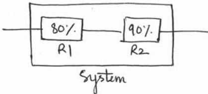
$$\begin{aligned} R_T &= R_1 \times R_2 \\ &= 0.8 \times 0.9 \\ &= 0.72 \\ &= 72\% \end{aligned}$$
