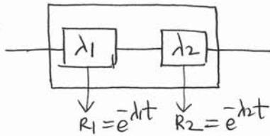
$$\begin{aligned} R_S &= R_1 \times R_2 \\ &= e^{-\lambda_1 t} \times e^{-\lambda_2 t} \\ &= e^{-(\lambda_1 + \lambda_2)t} \end{aligned}$$
