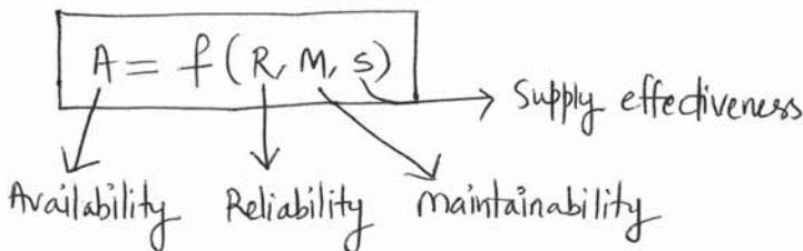
$$A = \frac{\text{MTBF}}{\text{MTBF} + \text{MTTR} + \text{MTWS}}$$
