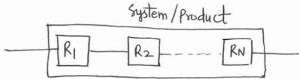
$$R_S = R_1 \times R_2 \times \dots \times R_N$$
